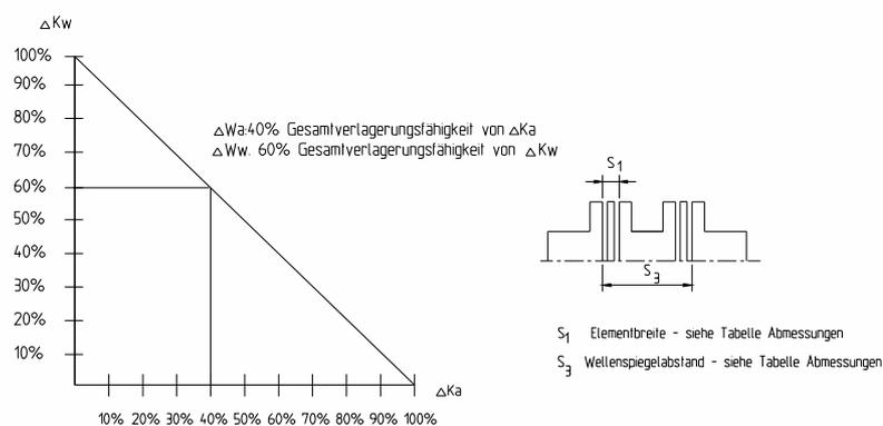
?Wa: 40% total displacement capacity of ?Ka
